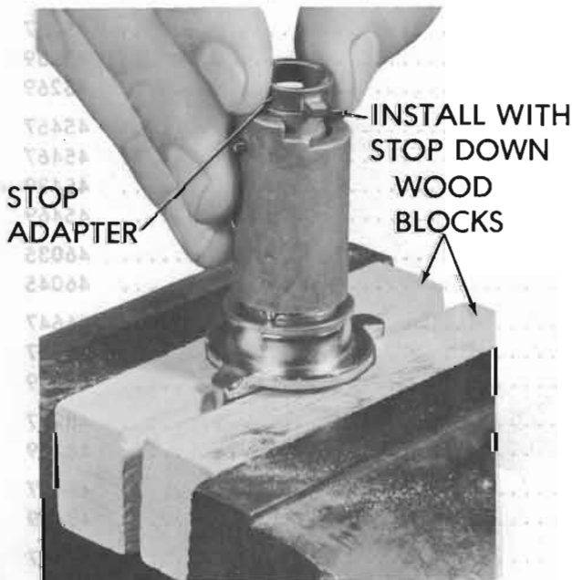
Figure 00-6 Installing Stop Adapter on Lock Cylinder
