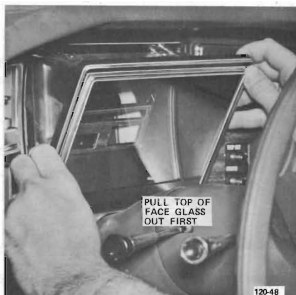
Figure 120-48 Removing Speedo Face Glass
