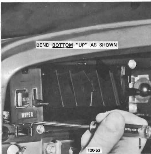
Figure 120-53 Removing Windshield Wiper Switch
