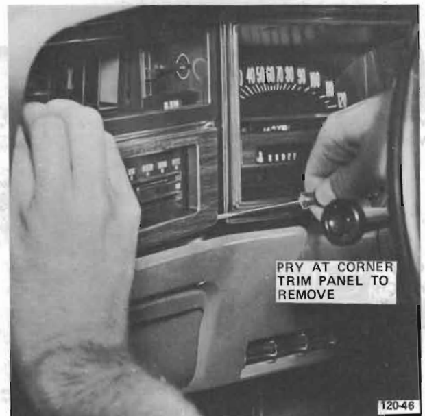
Figure 120-46 Removing Instrument Trim Panels
