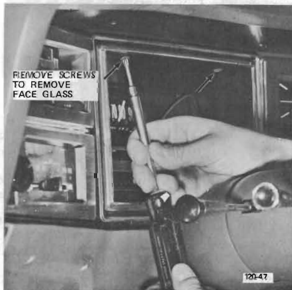
Figure 120-47 Speedo Glass Retaining Screws
