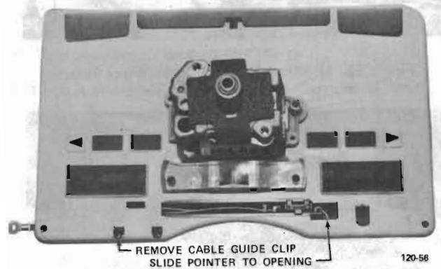
Figure 120-56 Removing Shift Indicator
