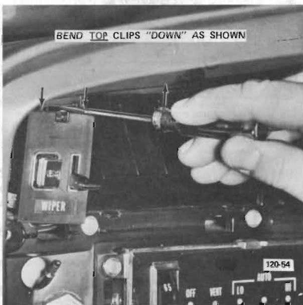
Figure 120-54 Removing Windshield Wiper Switch
