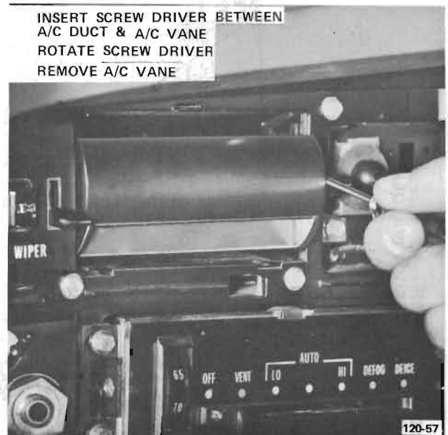
Figure 120-57 Removing A/C Outlet Vanes
