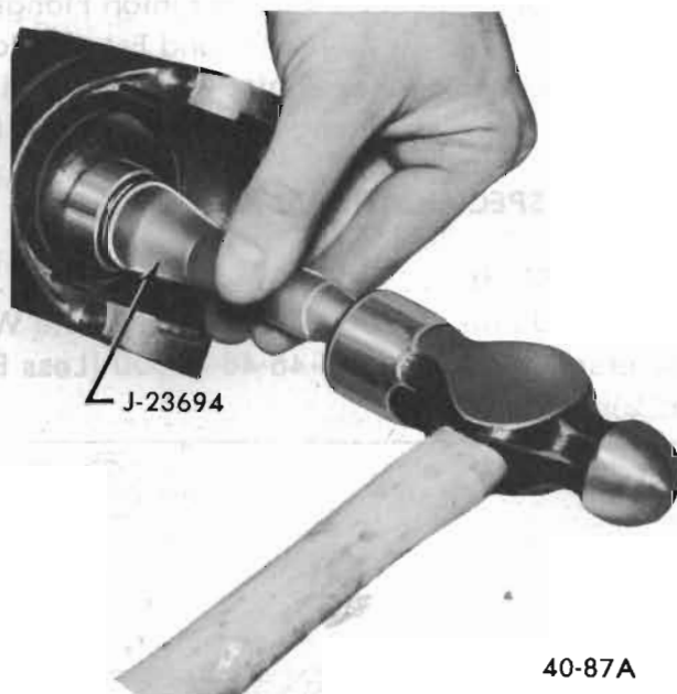
Figure 40-74 Installing Ball Stud Seal
