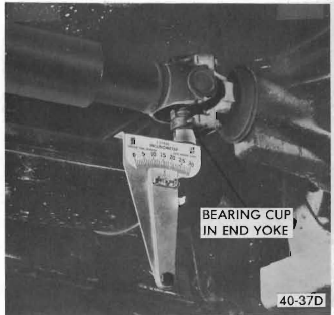
Figure 40-52 Measuring Angle at Rear of Propeller Shaft
