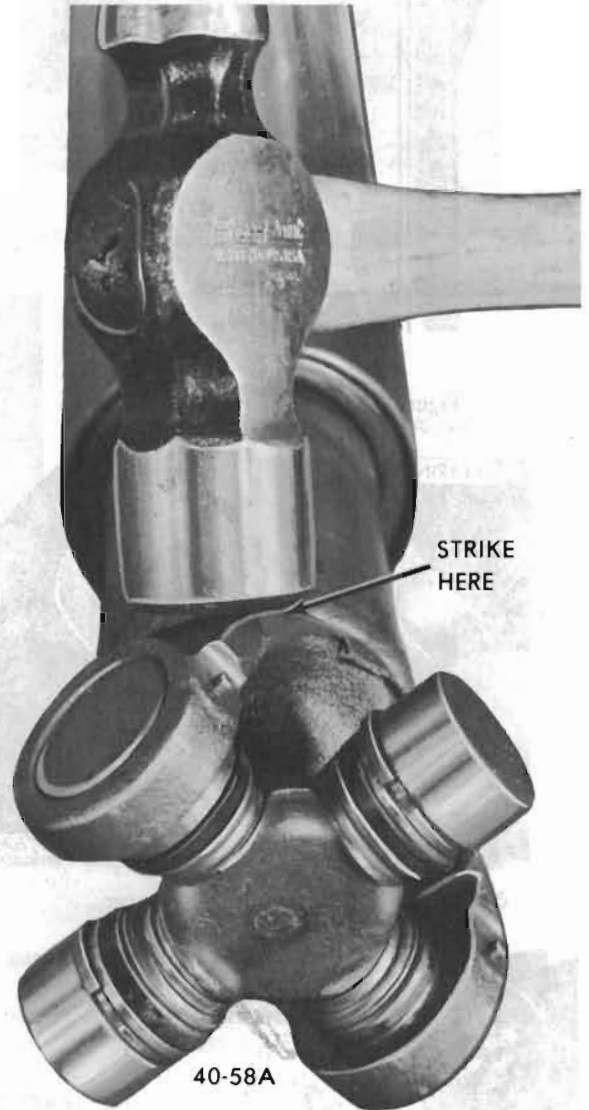
Figure 40-71 Seating U-joint Snap Rings
