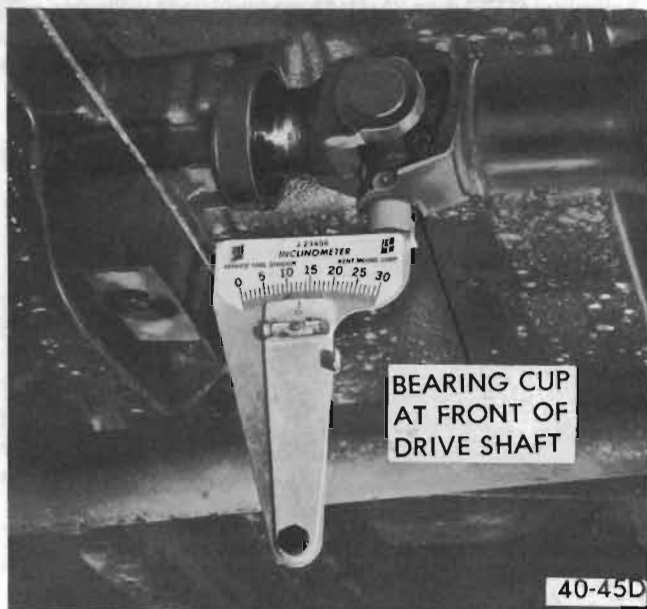
Figure 40-54 Measuring Angle at Front of Propeller Shaft
