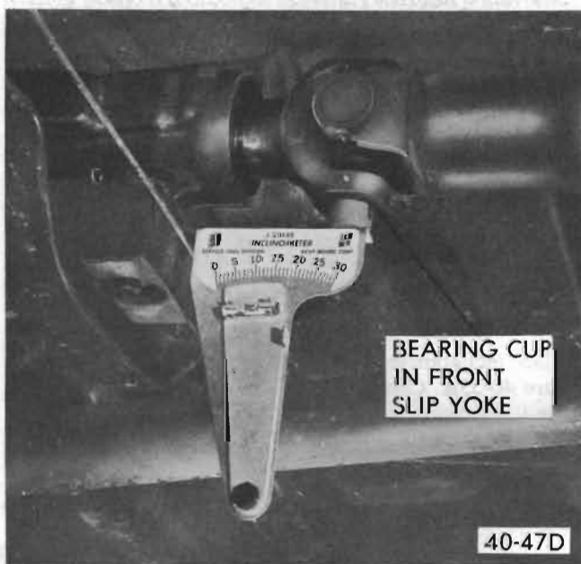
Figure 40-55 Measuring Angle at Front of Propeller Shaft
