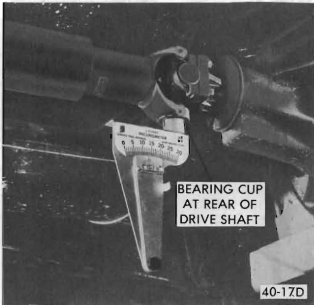
Figure 40-51 Measuring Angle at Rear of Propeller Shaft
