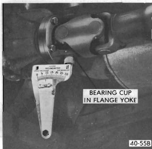
Figure 40-55B - Measuring Angle at Rear of Propeller Shaft
