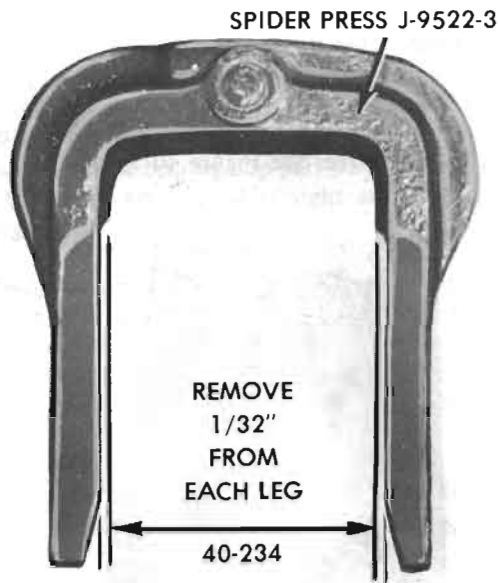
Figure 40-65 Spider Press Leg Rework
