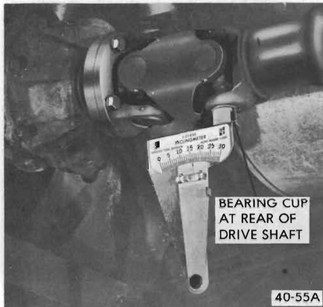
Figure 40-55A - Measuring Angle at Rear of Propeller Shaft
