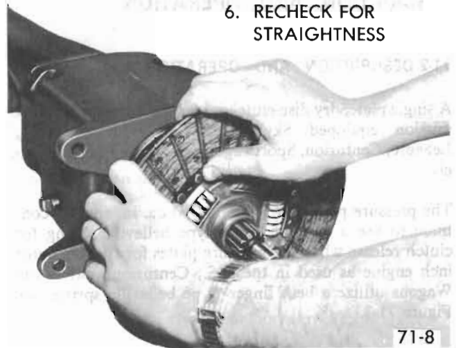
Figure 71-2 - Checking Driven Plate Run-Out
