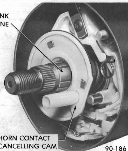
Figure 90-107 - Horn Contact - Cancelling Cam Installed
