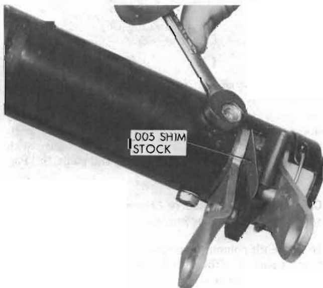
Figure 90-109 - Adjusting Shift Tube Bearing
