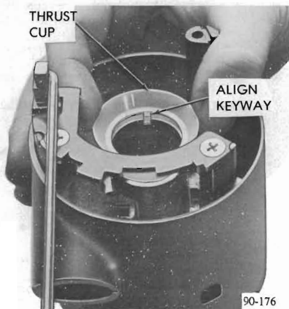
Figure 90-89 Removing or Installing Thrust Cup
