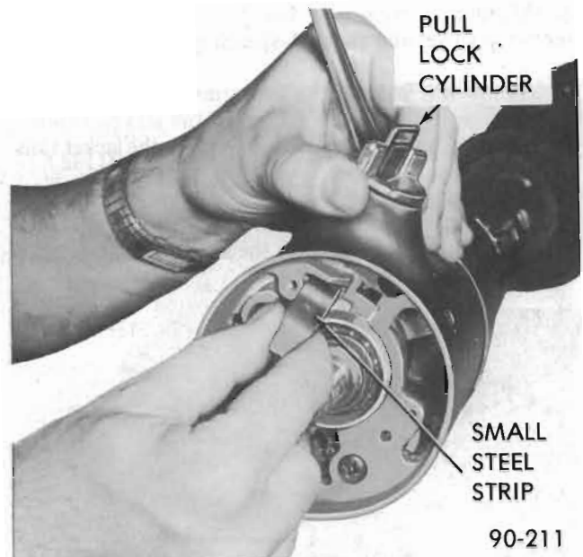
Figure 90-111 - Removing Ignition Lock Cylinder
