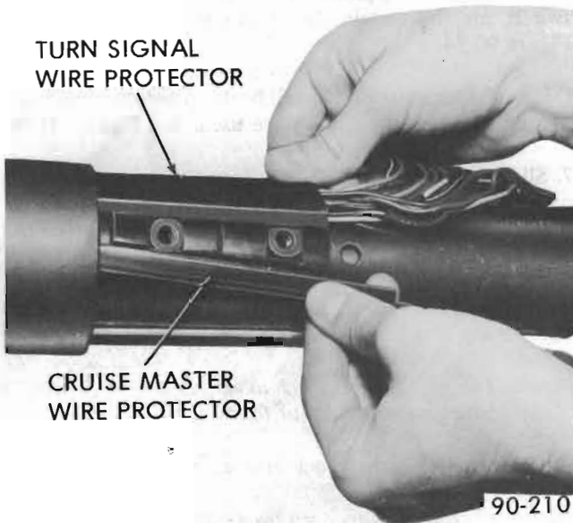
Figure 90-110 - Signal Switch Wire Protector
